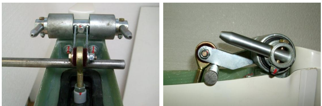
Fig. 4 Inspection of elevator control rod - apply a force to the stick
