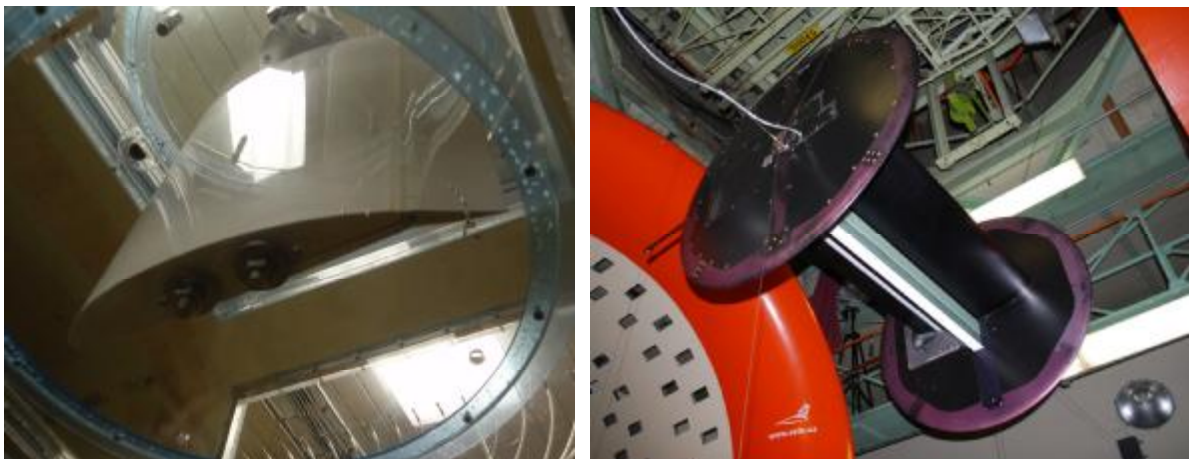
Wind-tunnel testing of TS airfoils: closed test section IT AS (left), open section (ARTI) with deployed dive brake
